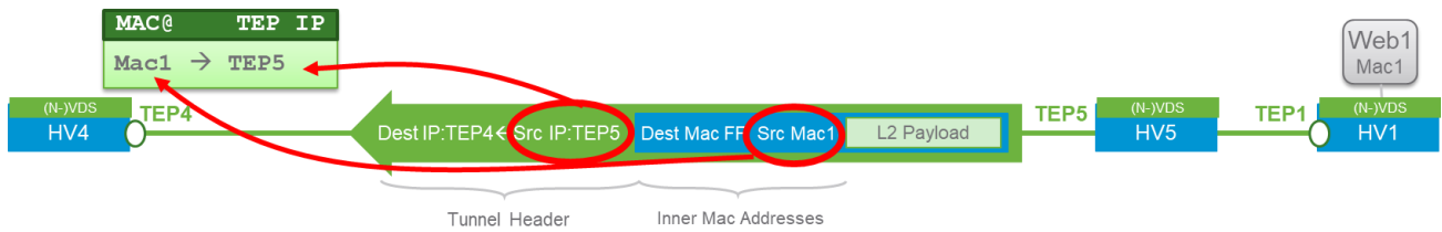
Figure 3-12: Data Plane Learning Using Tunnel Source IP Address
